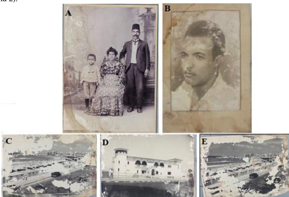
Fig. 1. Black and white photograph samples of the used private collection showing various signs of deterioration including, gelatin binder staining and losses
