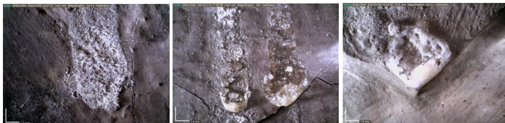
Fig. 4. Micrographs in raking light showing the “needle-shaped”, “cubic” and “amorphous” formations respectively
