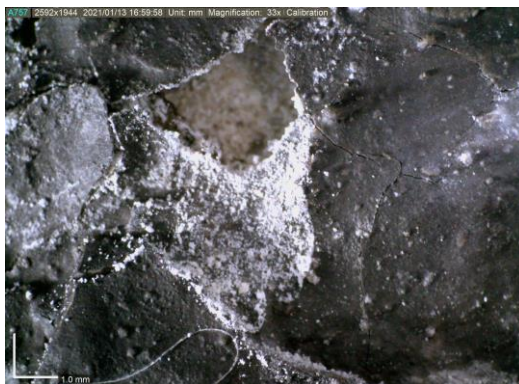
Fig. 3. Micrograph of drip emerging from a paint loss
